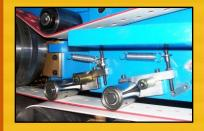
**Hold-Down Roller Kit** – Includes a complete vacuum-folding belt holddown roller assembly, roller with bearings, shaft, pivot shaft, jack screw, tee-nut fastener, spring, pivot plate and socket-head shoulder screws.
